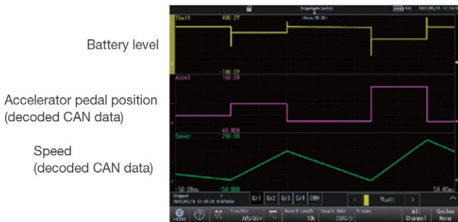
Figure 1 Display and recording of decoded bus traffic
